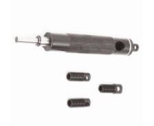
Our rivet removal tool is designed to keep the drill bit centered on the AN470 rivet head. The cupped drill guide also keeps the bit from slipping off and ruining the sheet metal around it. This tool is completely adjustable for drilling depth. It comes complete with four guides and drill bits for #3, #4, #5, and #6 rivets.
